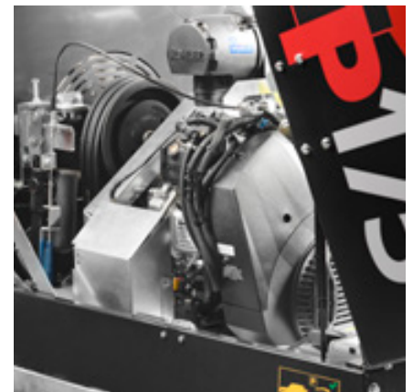
Powerful Kohler EFI engine with 38 HP
