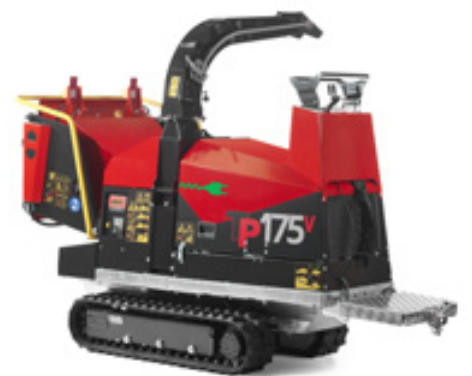
Manual control panel and platform with 20 kg safety switch as an option
