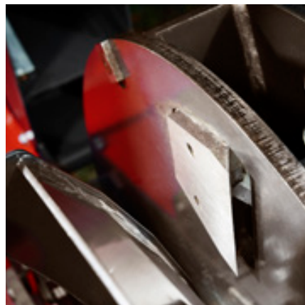
Displaced blades (2 pcs.) constantly engaging material
