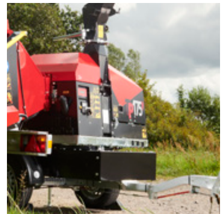
220° turntable is optional (increases weight by 80 kg)
