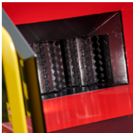
Vertical infeed rollers from TP forest design
