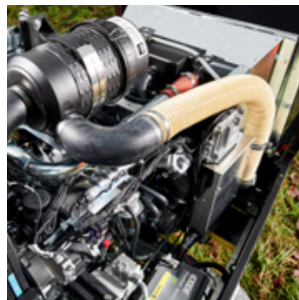
Hatz 4H50 Stage V engine with 55 kW
