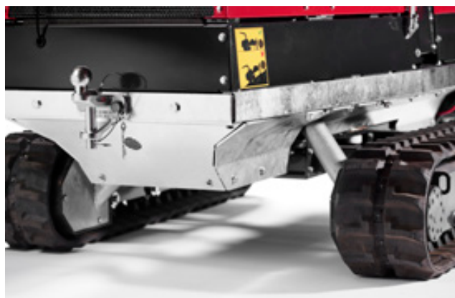
Ground clearance of 200 mm, easy service and reinforced hose protection. Variable track width 1,150-1,350 mm
