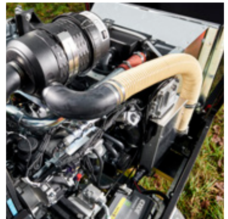
Motor Hatz 4H50 Stage V de 55,0 kW
